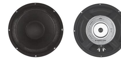
**17** Bass guitar driver for sealed or vented cabinets. Classic American bass guitar tone. Π Ferrite magnet, 8 ohm, 2" Copper Voice Coil, Stamped Frame, 200W.
