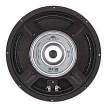
**0**<sup>11</sup> Medium power pro audio and MI driver. Works well as a mid in small sealed boxes, as a mid/bass driver in vented box, or for Bass Guitar in medium sized vented cabinets. Ferrite Magnet, Stamped Frame, 1.5" Copper Voice Coil, 125 Watts, 95.3db Sensitivity
