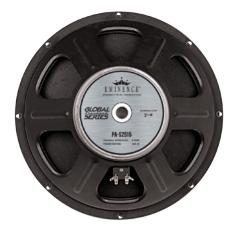
**15**" High power for pro audio and MI applications. Great for small sealed floor wedges or medium sized vented boxes for mains, monitors, or bass guitar. Ferrite Magnet, Stamped Frame, 2.5" Copper Voice Coil, 99.5dB Sensitivity, 300 Watts
