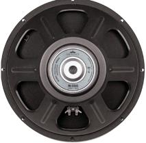
**15**" Medium power pro audio and MI driver. Works well in medium to large sealed cabinets, or in large vented cabinets. Ferrite Magnet, Stamped Frame, 1.75" Copper Voice Coil, 125 Watts, 97.7dB sensitivity
