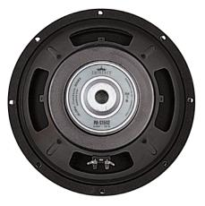
12" Medium power pro audio and MI driver. Works well as a mid in small sealed boxes, as a mid/bass driver in vented box, or for Bass Guitar in medium sized vented cabinets. Ferrite Magnet, Stamped Frame, 1.5" Copper Voice Coil, 125 Watts, 96.5dB
