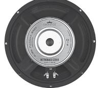
**4**-ohm version of our bass guitar driver for sealed or vented cabinets. Classic American bass guitar tone. 8 ohm, Ferrite magnet, 2" Copper Voice Coil, Stamped Frame, 200W.
