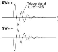
When the Polarity Switch is set to the "+" position, the trigger signal will begin on the positive side of the ground level.
