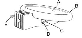
As shown below, you can attach the PD-7 or PD-9 to a drum stand in two different ways. To change the angle for inserting the rod, first loosen the Stand Fixing Screw and then rotate the eyebolt by degrees.
