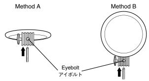
NOTE If you use method B, do not try to insert the rod into the eyebolt by force, as it will not go any further than a predetermined point.
