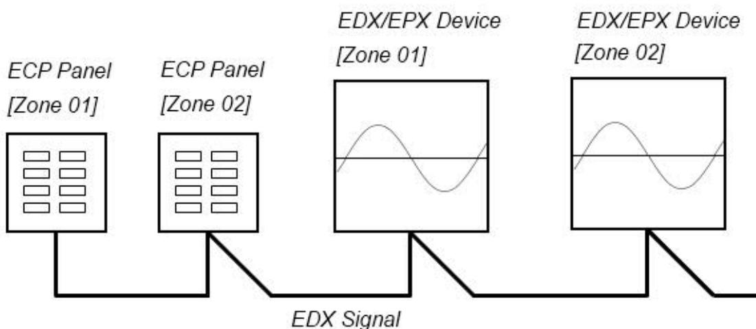
ECP scene panel 1 controls EDX/EPX device 1.
