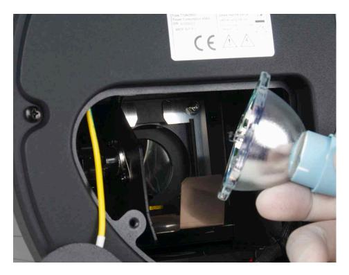
**6.** Using a clean cloth or gloves, gently install the new lamp into the fixture using your thumb and index finger, making sure the spade terminals on the base of the lamp are facing straight **UP**.
